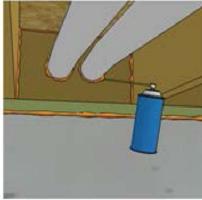
Figure CSTFx. Foam sealant at band joist insulation and penetrations
