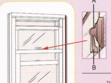
To open, simply disengage the lock (A) by pushing on the thumb lever (B). When disengaged, both sashes (C) will be free to move up or down.
