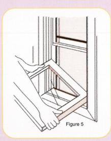
Each sash can be completely removed for glass replacement, balance service, or screen removal. Use caution when removing the sashes as they are heavy.
