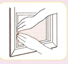
Each screen is fitted with a rail or tabs on one side which, when pushed to the opposite side, will compress the screen springs into the side channel and allow the screen to be removed as shown.
